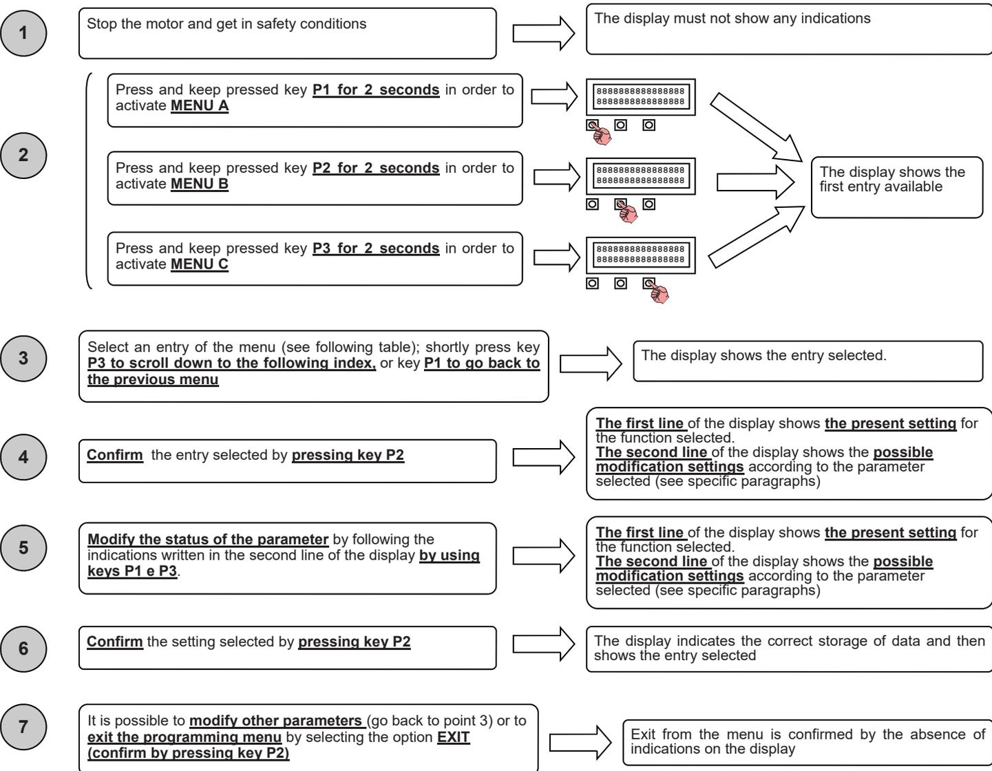
AUTOMATIC EXIT FROM THE MENU: the menu exits automatically in case of long inactivity (longer than 15 seconds)
