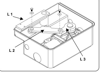
Insert the ball in the pin located on the box and fit the gate anchorage lever (L1)
