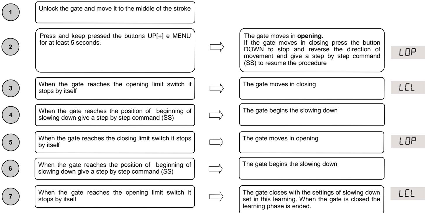
**Warning:** in case of intervention of a safety device, the learning is stopped and will appear on the display the written L--. Press Step by Step button to start again the learning from the 2<sup>nd</sup> point.
