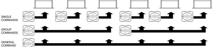
Each roller shutter can be operated by many B.RO WALL transmitters, up to 1000.- The transmitter can be recorded with roller shutter receiver through the learning modality shown in the instructions of the receiver.
