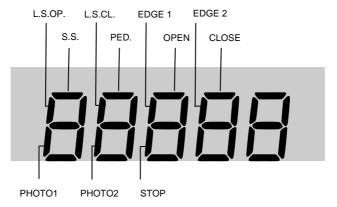
N.B. The lit segments indicate that the input is activated.
