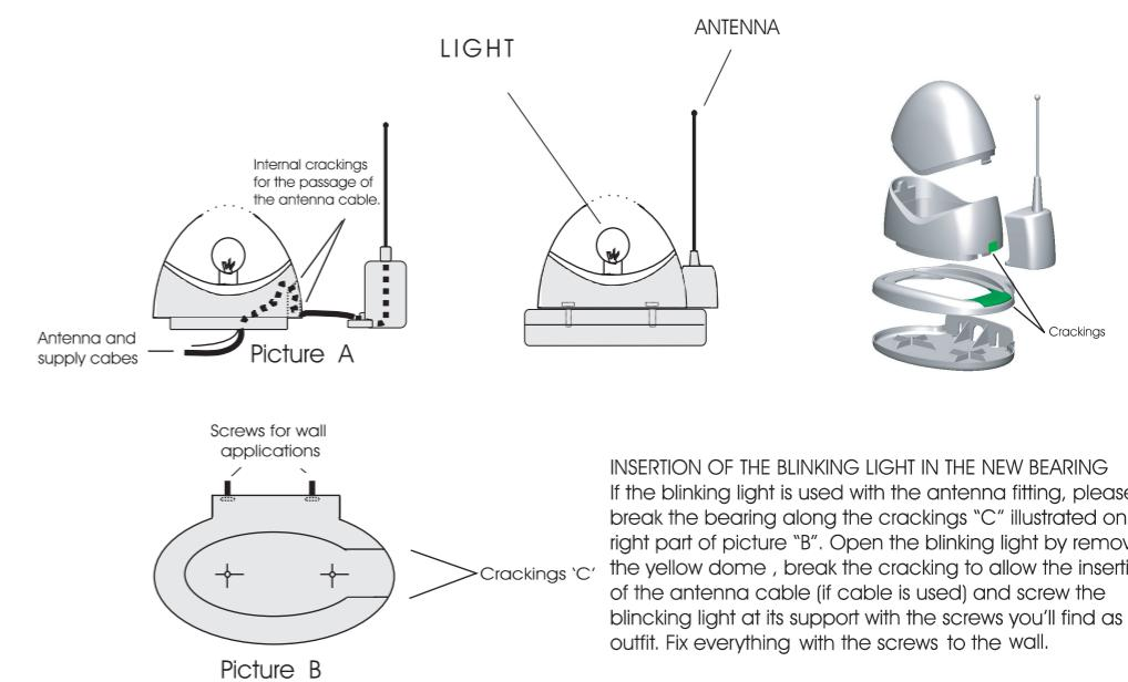
Antenna fitting is available for both models and for frequency 30.875 - 40.665 - 300 - or 433.92 Mhz; the initials are: AL30, AL40, AL300, AL433. For insertion of antenna cable (if it is used) see picture A.
