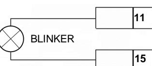
Connect an eventual blinker with self-blinking circuit between clamps L 11 (line in) and N 15 (common of the motor).
