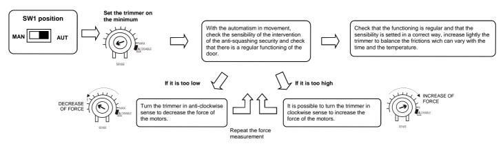
Warning: With the trimmer in disabled position (flashing light turn on), the anti-squashing security is excluded.
