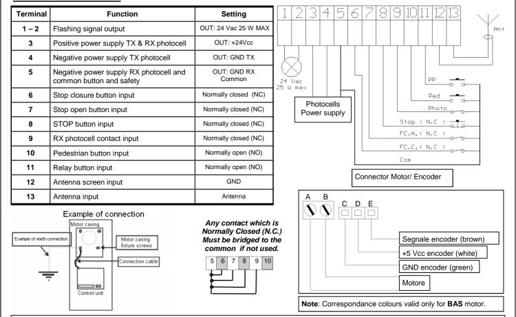
IMPORTANT: to obtain a correct working of the accessories (photo devices in particular) connected to the control box, is very important that the entire system (motor+ control box) has a single mass reference system. You must therefore connect a small cable between the motor casing and the control box at the point shown in the figure. If there is a good ground connection it is advisable to connect it to the system.
