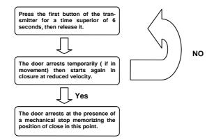
Warning: During the operation of resynchronization, the intervention of the anti-squashing security is interpreted like identification of the closing position. To avoid the volontary intervention the sensibility of the self results remarkably reduced respect to the conditions of normal functioning.
