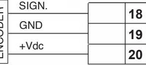
Connect the encoder's SIGN cable to clamp 18 of the terminal board.
