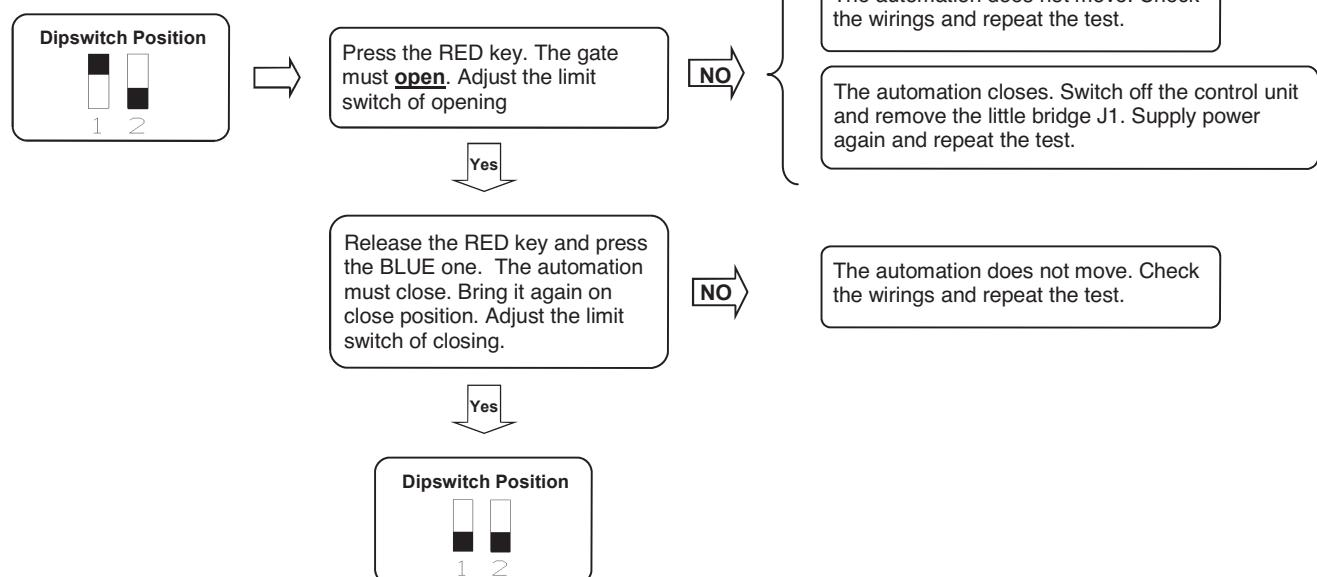
Warning: the removing of JUMPER 1 must be carried out with control unit switched off. As soon as the control unit switches on again, the motor rotation sense and the limit switches inputs are automatically inverted. It is advisable to check the correct functioning of the limit switches with the operations above described.
