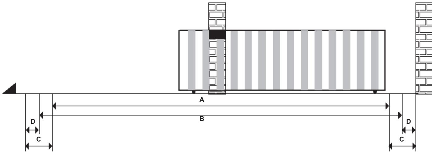
A= Intervention zone of the amperometric sensor with movement inversion
