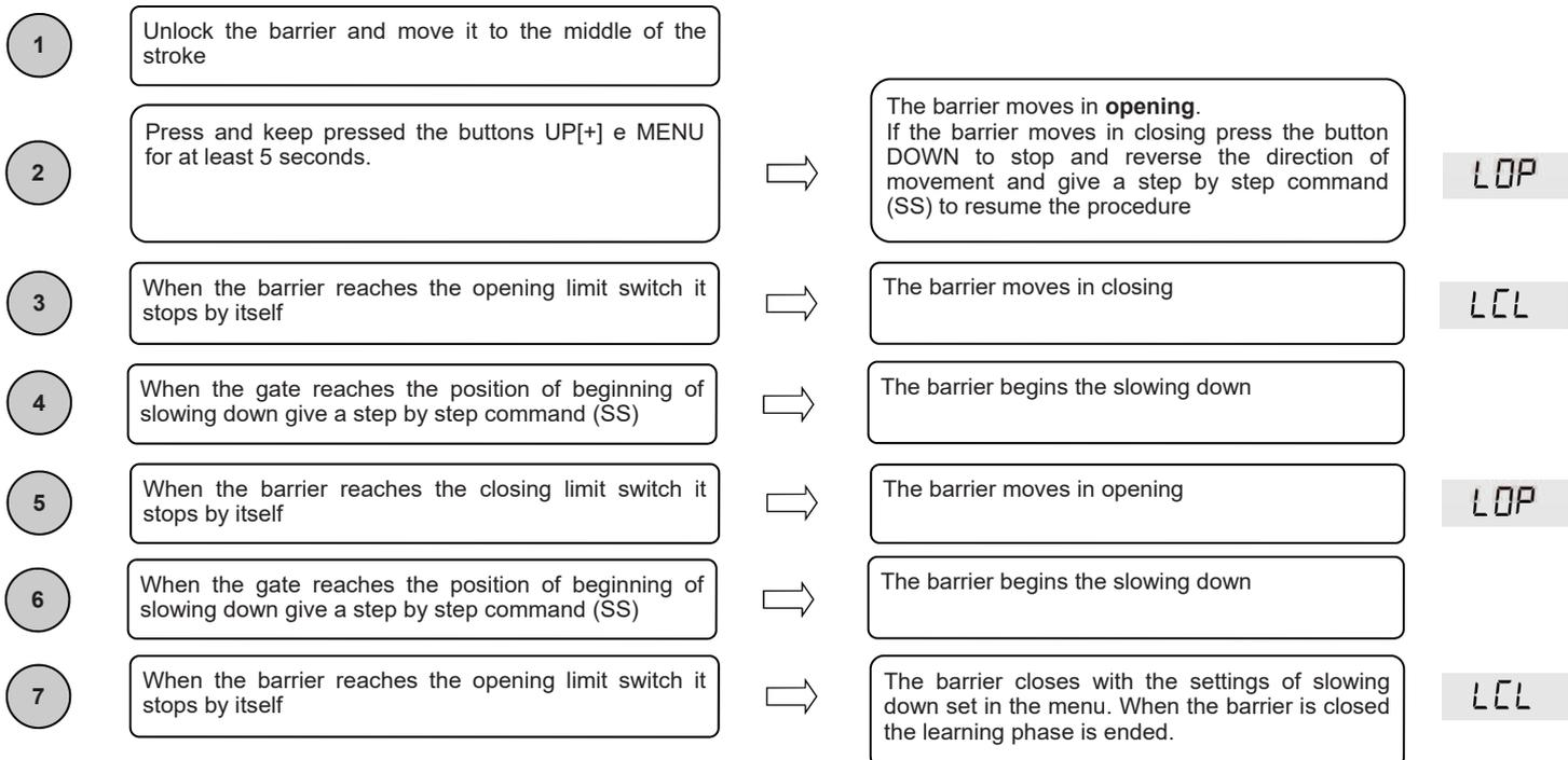
**Warning:** in case of intervention of a safety device, the learning is stopped and will appear on the display the written Press Step by Step key to start again the learning from the 2<sup>nd</sup> point.
