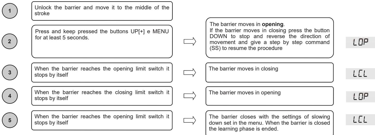
**Warning:** in case of intervention of a safety device, the learning is stopped and will appear on the display the written Press Step by Step key to start again the learning from the 2<sup>nd</sup> point.
